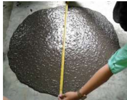
Fig. 2. Slump flow of HVFA-SCC of about 700 mm
