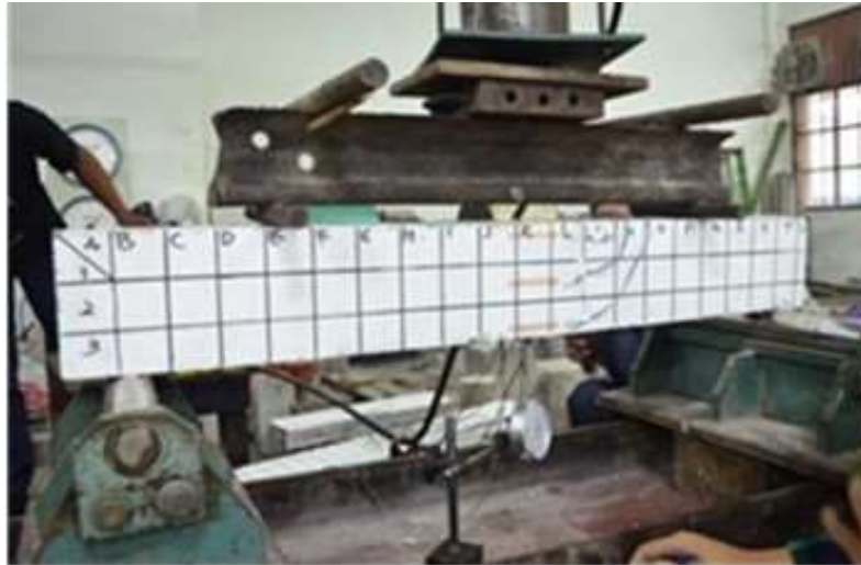
Fig. 4. Flexural strength test of RC beam
